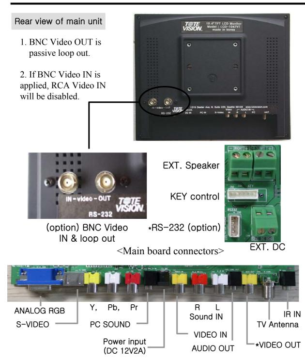
**\*VIDEO OUT** is active output for VCR recording for TV or composite video input. This can be used for a diversity antenna. If S-Video or component input is selected, display of this output will be changed to black and white because the color of the original input signal is already separated. In PC mode you will get TV signal.
